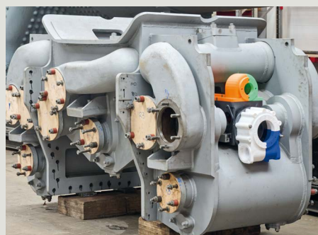
The 3D printed cambox in place, ready for testing at Darlington Locomotive Works.
